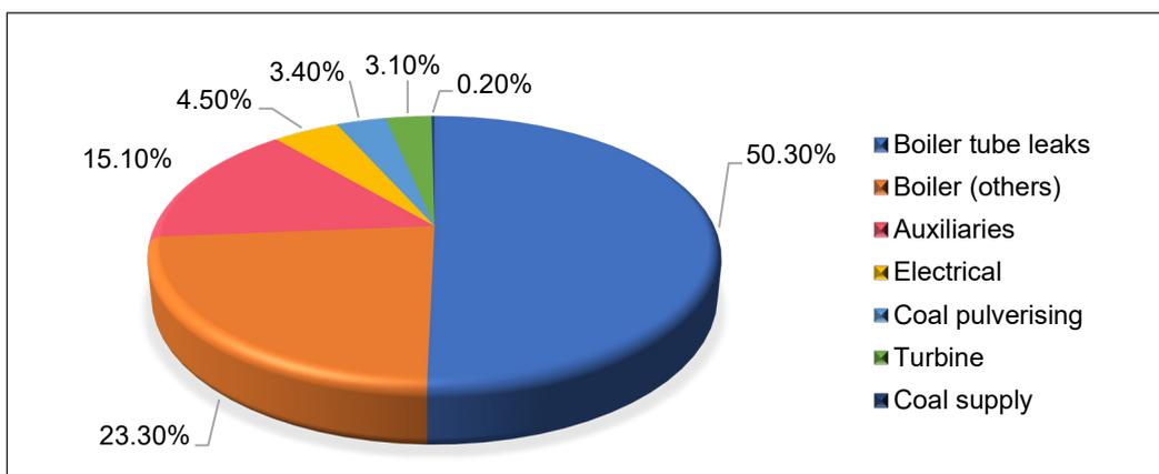
Figure 1. Main plant system contributor to power unit fault (2012 to 2020)
