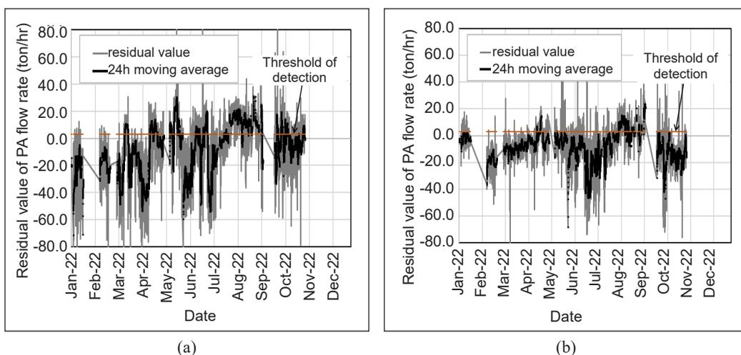
Figure 14. The residual value of total primary airflow and its 24-hour moving average in the year 2021 for: (a) model trained with 2012 to 2020 data; (b) model retrained with 2012 to 2021 data
