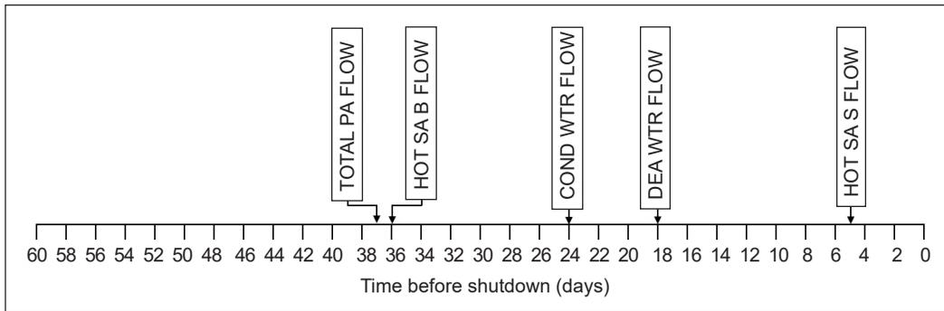
Figure 16. Sequence of boiler tube leak detection time by the corresponding models' residuals for Fault #14
