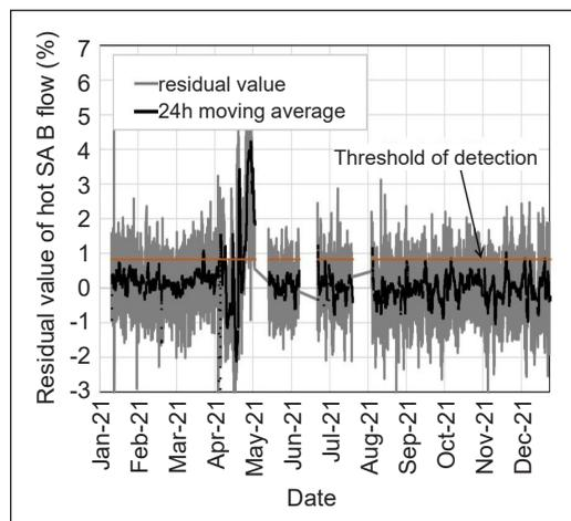
Figure 11. The residual value of hot secondary air B flow and its 24-hour moving average for the year 2021
