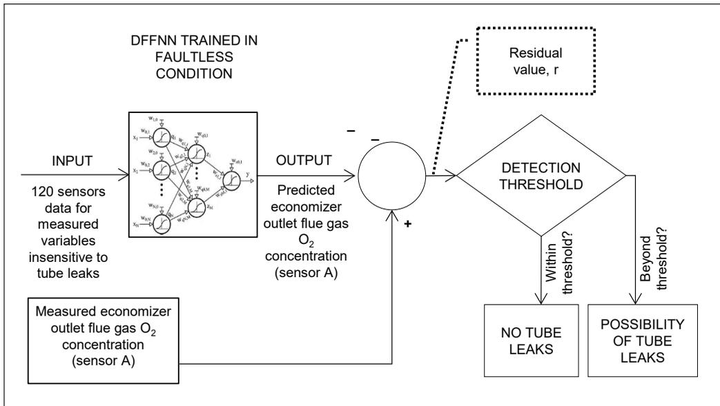
Figure 4. Example of economiser outlet flue gas O<sub>2</sub> concentration model for fault detection by residue method
