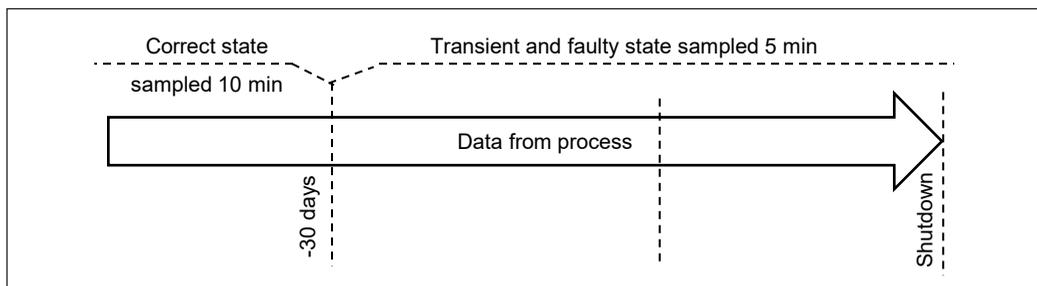
Figure 3. Data division before boiler emergency shutdown
