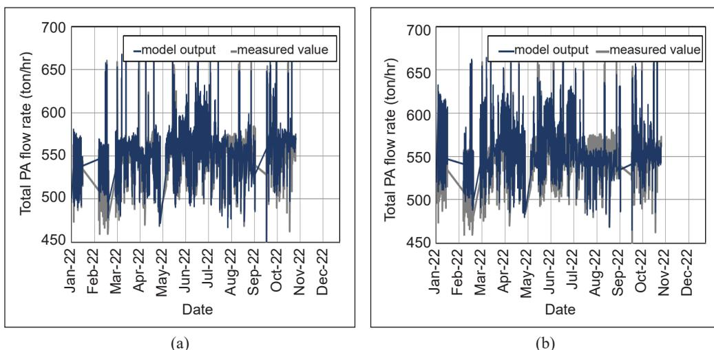
Figure 13. Measured value and output from TOTAL PA FLOW model in the year 2022 for: (a) model trained with 2012 to 2020 data; and (b) model retrained with 2012 to 2021 data
