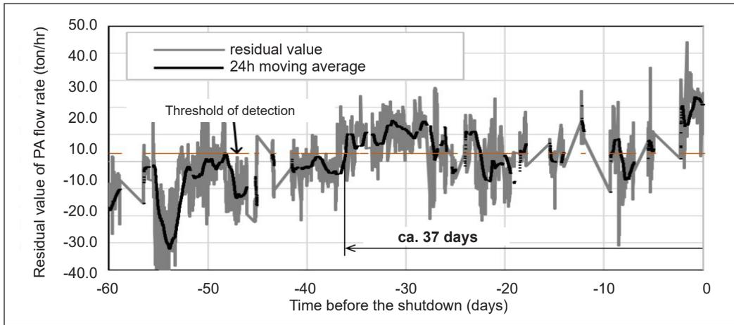
Figure 15. The residual value of total primary airflow and its 24-hour moving average for tube leak Fault #14
