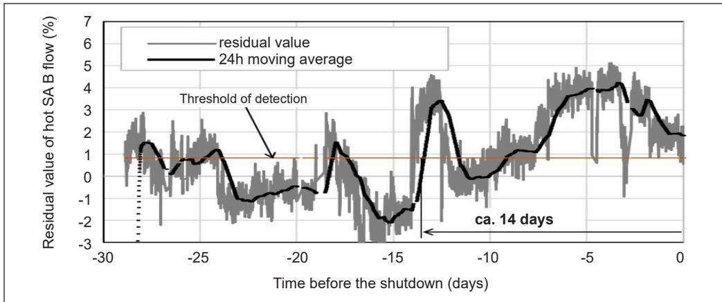
Figure 12. The residual value of hot secondary air B flow and its 24-hour moving average for tube leak Fault #13
