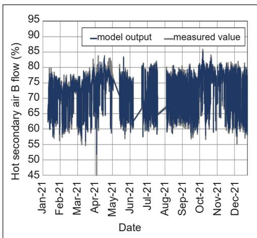
Figure 10. Measured value and output from the HOT SA B FLOW model for the year 2021
