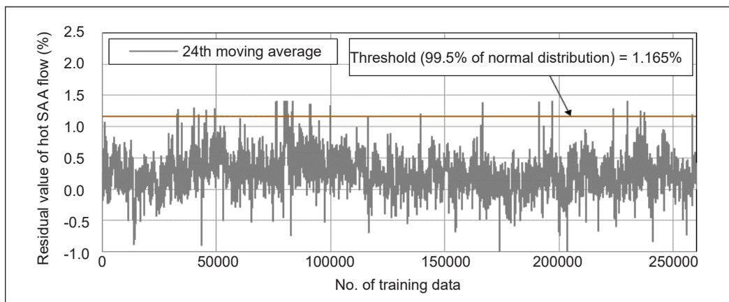
Figure 5. Determination of threshold of the detection limit for the residual value of hot secondary air A flow
