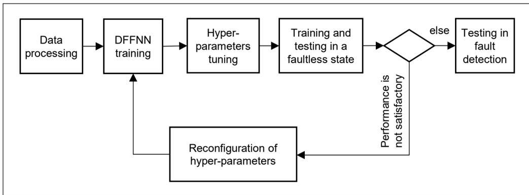
Figure 2. The algorithm for finding the best structures of DFFNN for fault detection
