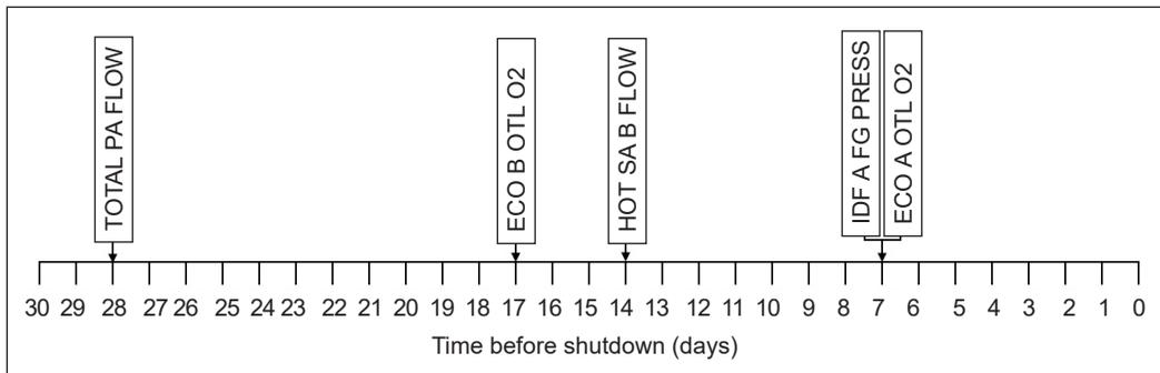
Figure 9. Sequence of boiler tube leak detection time by the corresponding models' residuals for Fault #13
