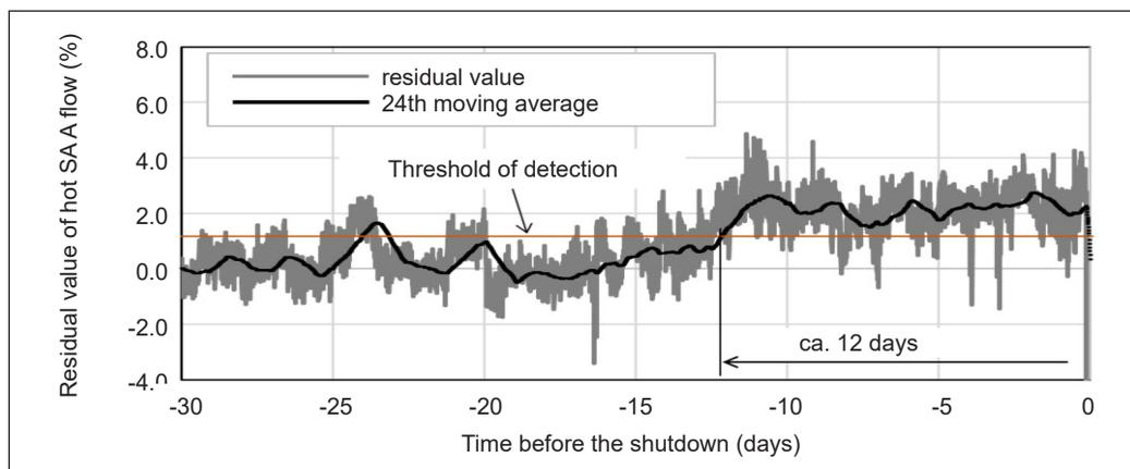
Figure 7. The residual value of hot secondary air A flow and its 24-hour moving average for tube leak Fault #10
