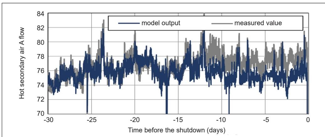
Figure 6. Exemplary courses of hot secondary air A flow, measured value and output from DFFNN model prior to shutdown of a boiler for tube leak Fault #10
