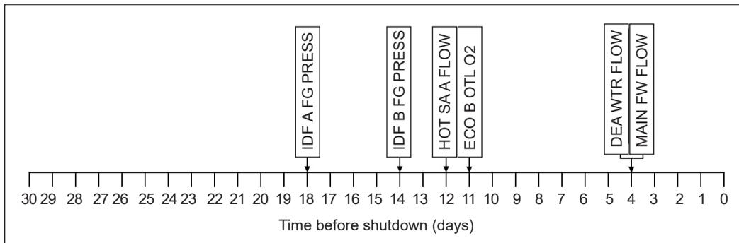
Figure 8. Sequence of boiler tube leak detection time by the corresponding models' residuals for Fault #10
